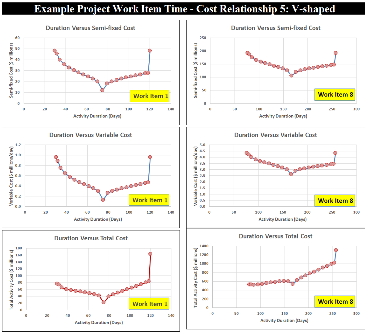
Fig S-7. Time-cost trends for work items 1 and 8 of example project for time-cost relationship 5. V-shaped .
